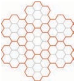
Construction of 7×7 wire rope.
