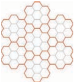
Construction of 7x7 wire rope.
